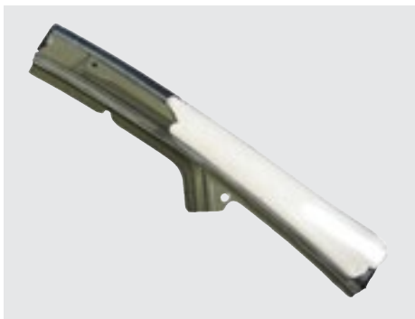
BETAFOAM™ Renue fills cavity space in a pillar application.
