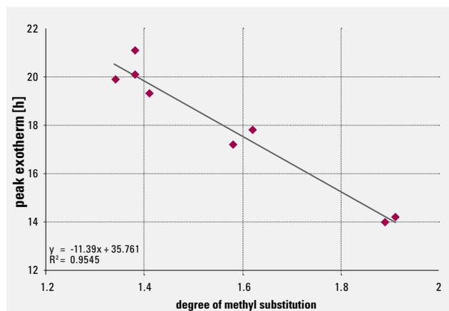
**Figure 9:** Linear Relationship of HEMC DS Methyl and the Peak Exotherm
