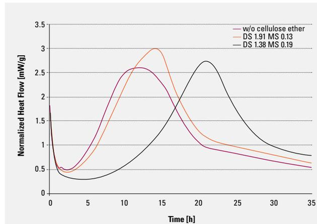
**Figure 8:** Heatflow Curves of Cement Setting Reaction with and without the Addition of HEMC's
