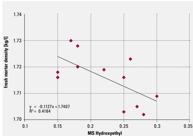
**Figure 3:** Plot of Fresh Mortar Density as a Function of MS Hydroxyethyl Substituents
