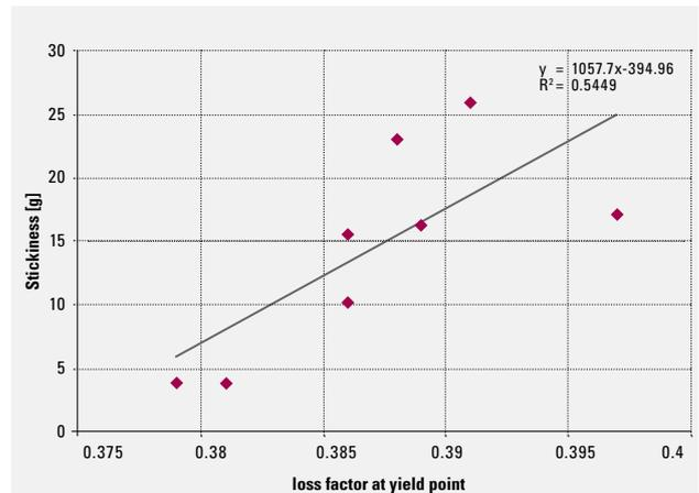
**Figure 6:** Plot of Loss Factor at Yield Point against Mortar Stickiness
