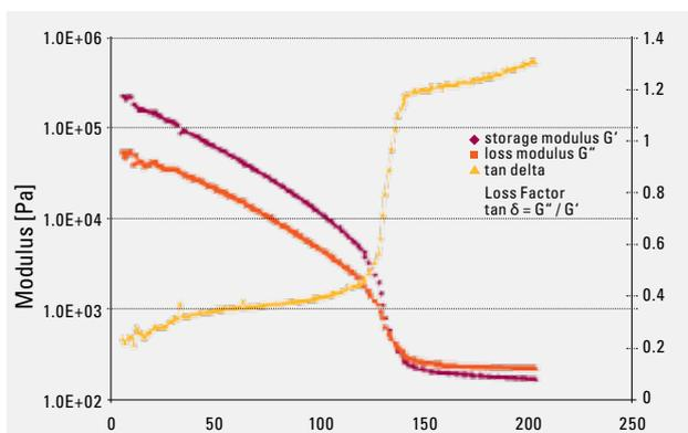
**Figure 5:** Plot of  $G'$ ,  $G''$  and  $\tan \delta$  as a Result of an Oscillating Amplitude Sweep of a Cement Render
