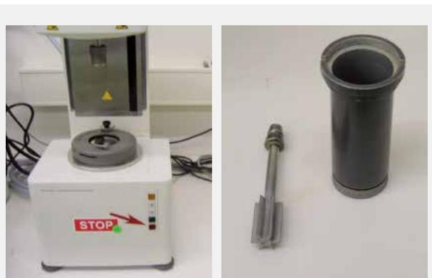
**Figure 4:** Oscillation-Rheometer for Mortar Systems
