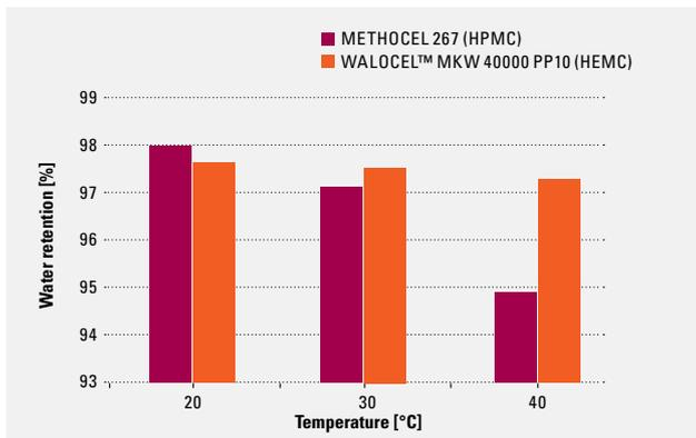
**Figure 2:** Water Retention of two Cellulose Ethers as a Function of Temperature
