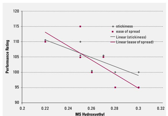
**Figure 7:** Plot of Plaster Performance Rating Against MS Hydroxyethyl
