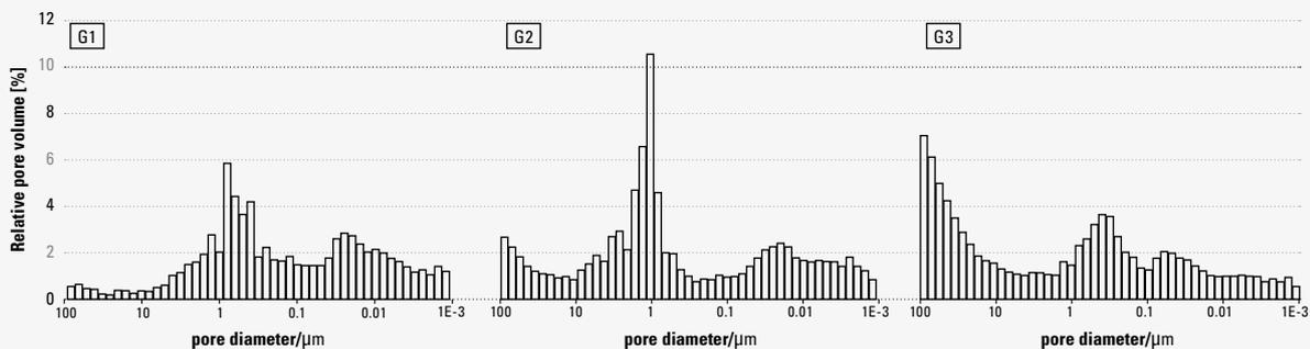
**Figure 6:** MIP – Pore size distribution in mortar
