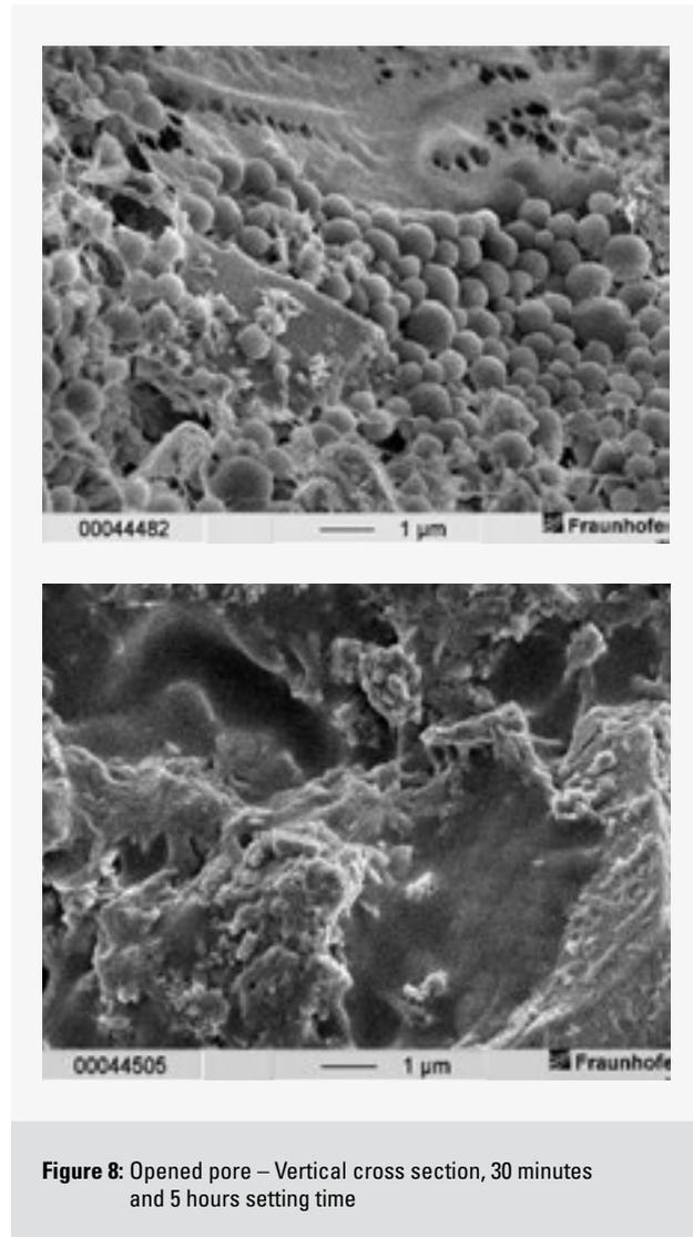
After 5 hours setting time the pore surface is complete covered with a latex film. The RDP particle structure is not visible anymore.
