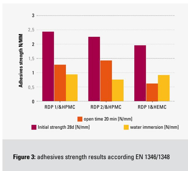
**Figure 3:** adhesives strength results according EN 1346/1348
