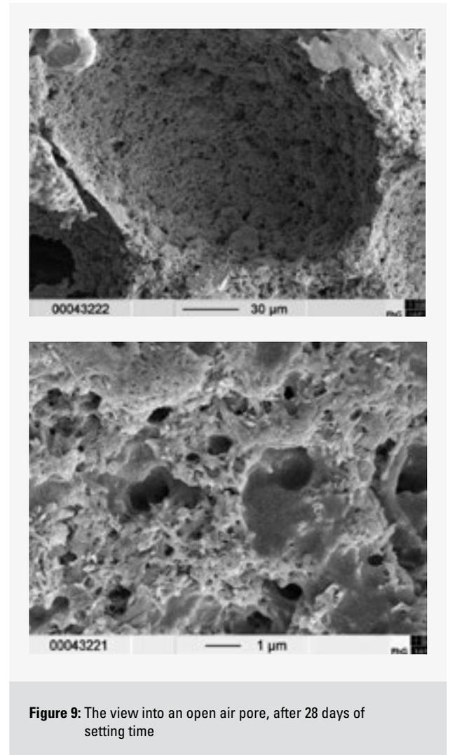
The SEM photograph of an air pore of a mortar which has cured for 28 days illustrates its complex structure. The growing crystals as a result of the cement hydration reaction have thoroughly penetrated the latex film and cover completely the interior side of the air pore.
