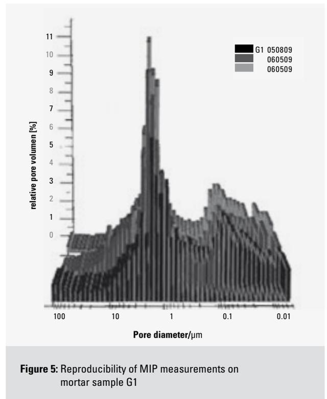
**Figure 5** shows the pore size distributions of three different measurements of mortar sample G1. Two distinct peaks at about 1.5  $\mu\text{m}$  and 0.08  $\mu\text{m}$  could be detected. The biggest portion of pore volume in the dried mortar samples consists of small capillary pores. The pore volume contribution of air pores (diameter > 6  $\mu\text{m}$ ) is relatively small.
