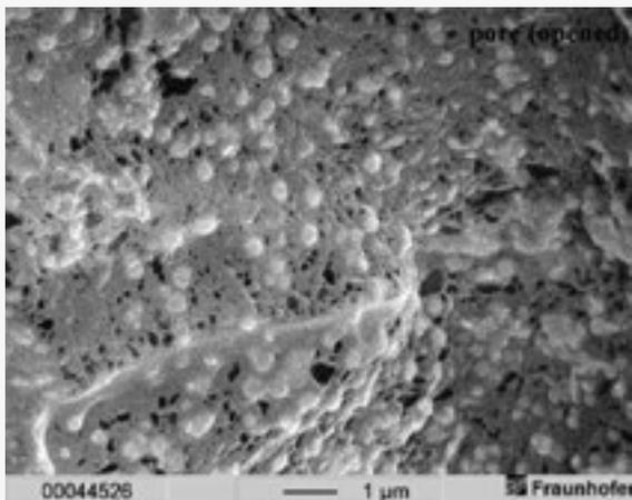
**Figure 10:** Mortar sample after 28 days of setting, re-wetted in water for 24 hours
