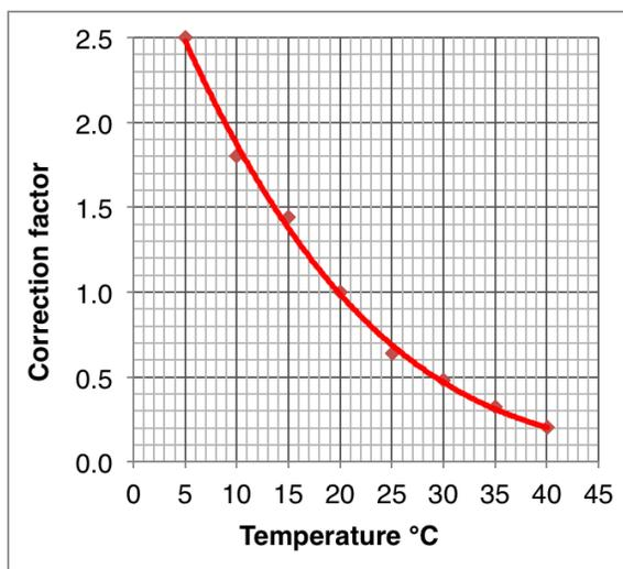
For instance, if a resin can accept a chlorine content of 0.2 mg/L at 20 °C, it should not be submitted to more than 0.1 mg/L at 30 °C (factor 0.5). If the temperature exceeds 40 °C, the tolerated concentration of oxidants is virtually zero.
