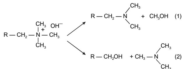
Reaction (1) converts the SBA into a WBA, producing methanol as a by-product, and reaction (2) converts the ammonium group to an alcohol, which has no ion exchange capability, and produces trimethylamine as a by-product.
