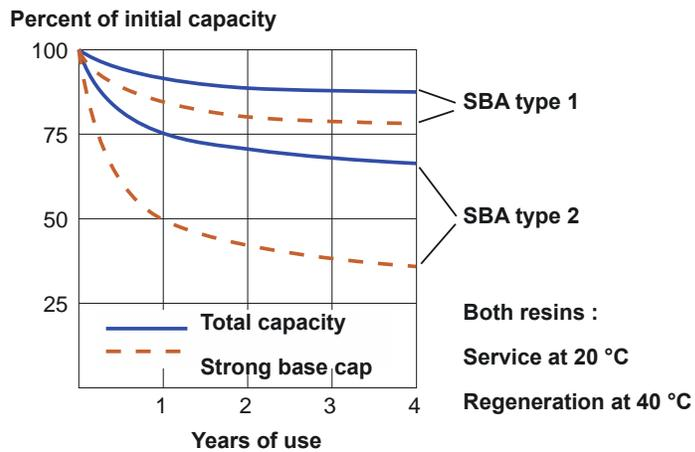
A faster degradation of the type 2 resin is clearly visible. For this reason, type 2 SBA resins should only be regenerated at ambient temperature.
