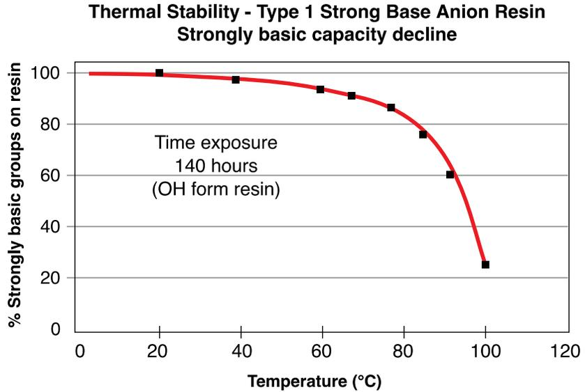
While styrenic type 1 anion exchange resins have the highest resistance to temperature compared to other strong base anion resins, capacity degradation still accelerates as temperature increases. For this reason, increasing operating temperature will always increase resin degradation rate.
