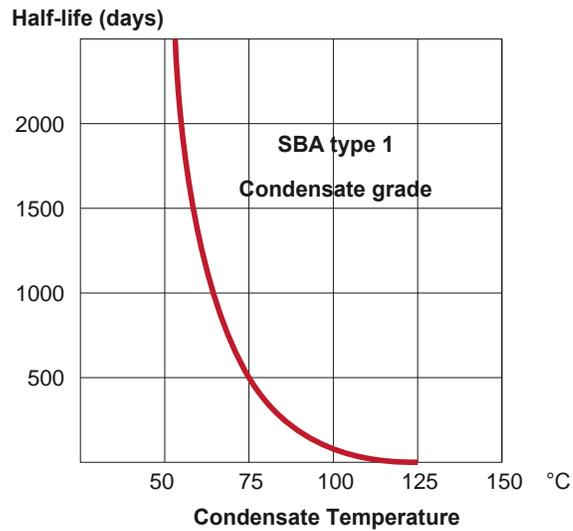
The half-life time is the time during which the resin loses half of its capacity.
