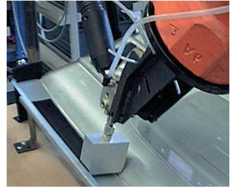
BETAMATE structural adhesives can be applied robotically in bead, swirl or jet spray using standard industrial equipment. The adhesives also can be applied manually from dispensing systems or cartridges.
