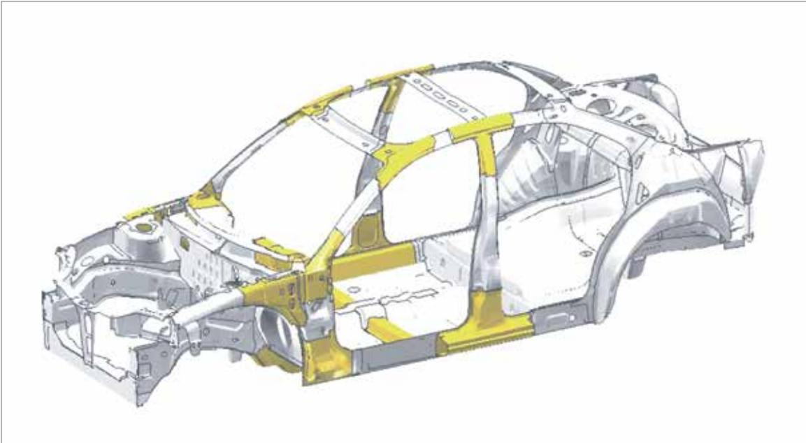
Figure 7 - Structural foam applications to the vehicle body.
