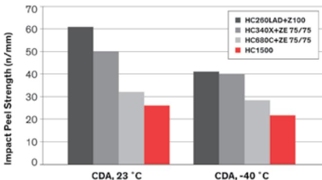
Figure 3a - Impact peel strength depending on steel grades and test temperatures.
