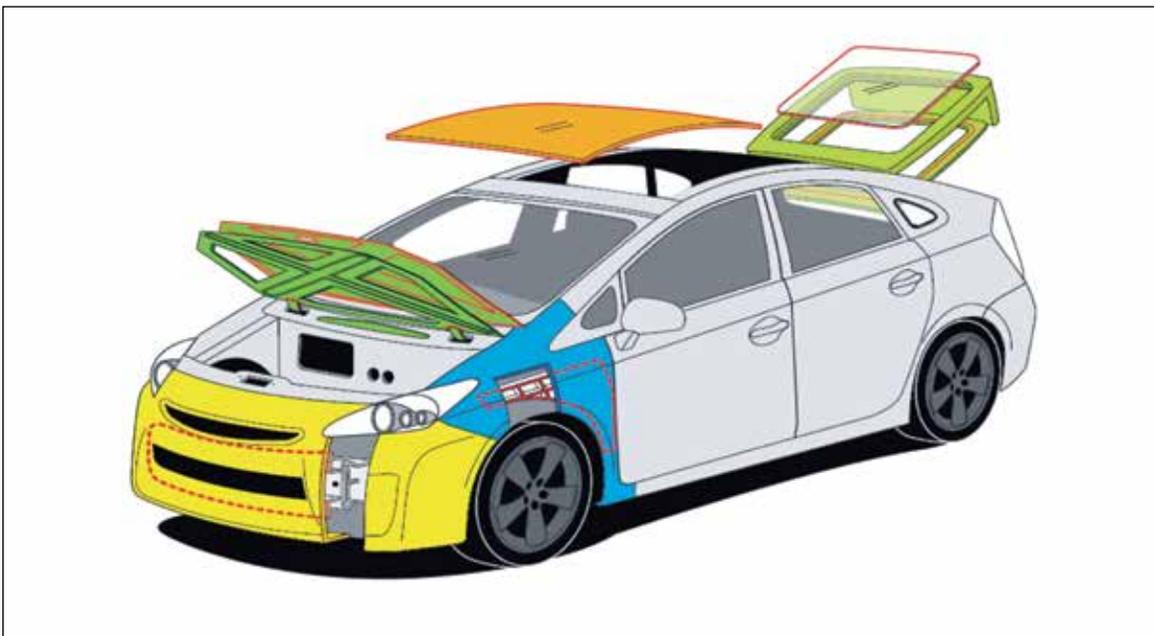
Figure 2 - Potential application areas of bonded hybrid composites.
