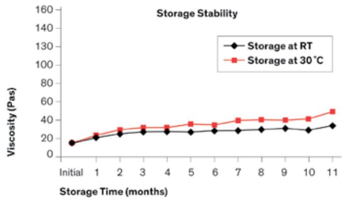
Figure 4 - Viscosity increase over time.
