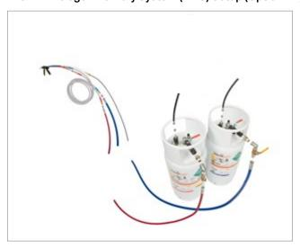
NOTE: (Optional) Dry nitrogen is used for pressurizing the FROTH-PAK™ ULTRA Premium Foam Insulation System and is not supplied. It may be obtained for a nominal rental charge from any local welding supplier. Order standard size (industrial grade) cylinder with CGA 580 nitrogen fitting. Refer to FROTH-PAK™ ULTRA Premium Foam Insulation System Installation drawing, page A2.
