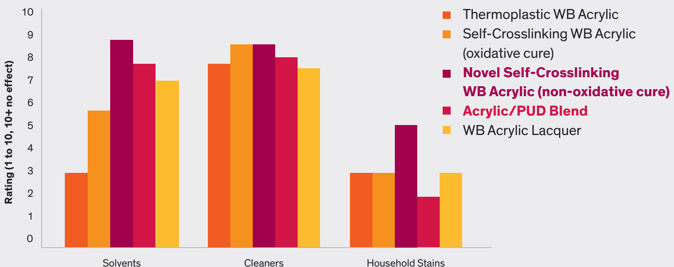
Fig.1. Systems based on novel self-crosslinking acrylic resin (non-oxidative) demonstrate good chemical resistance compared to other water-based systems.
