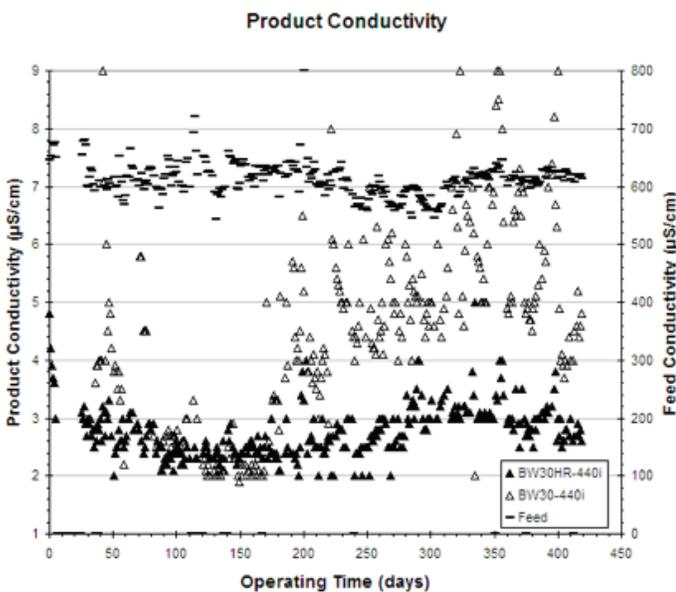
Figure 2: Product conductivity for the first year of operation.
