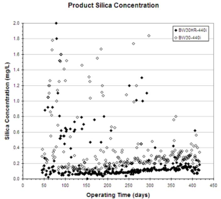
Figure 3: Product silica concentration for the first year of operation.
