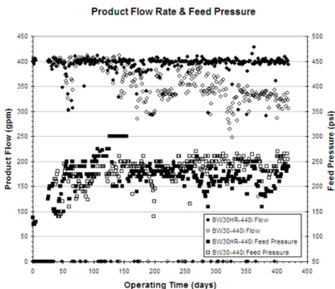
Figure 1: Product flow and feed pressure for the first year of operation.
