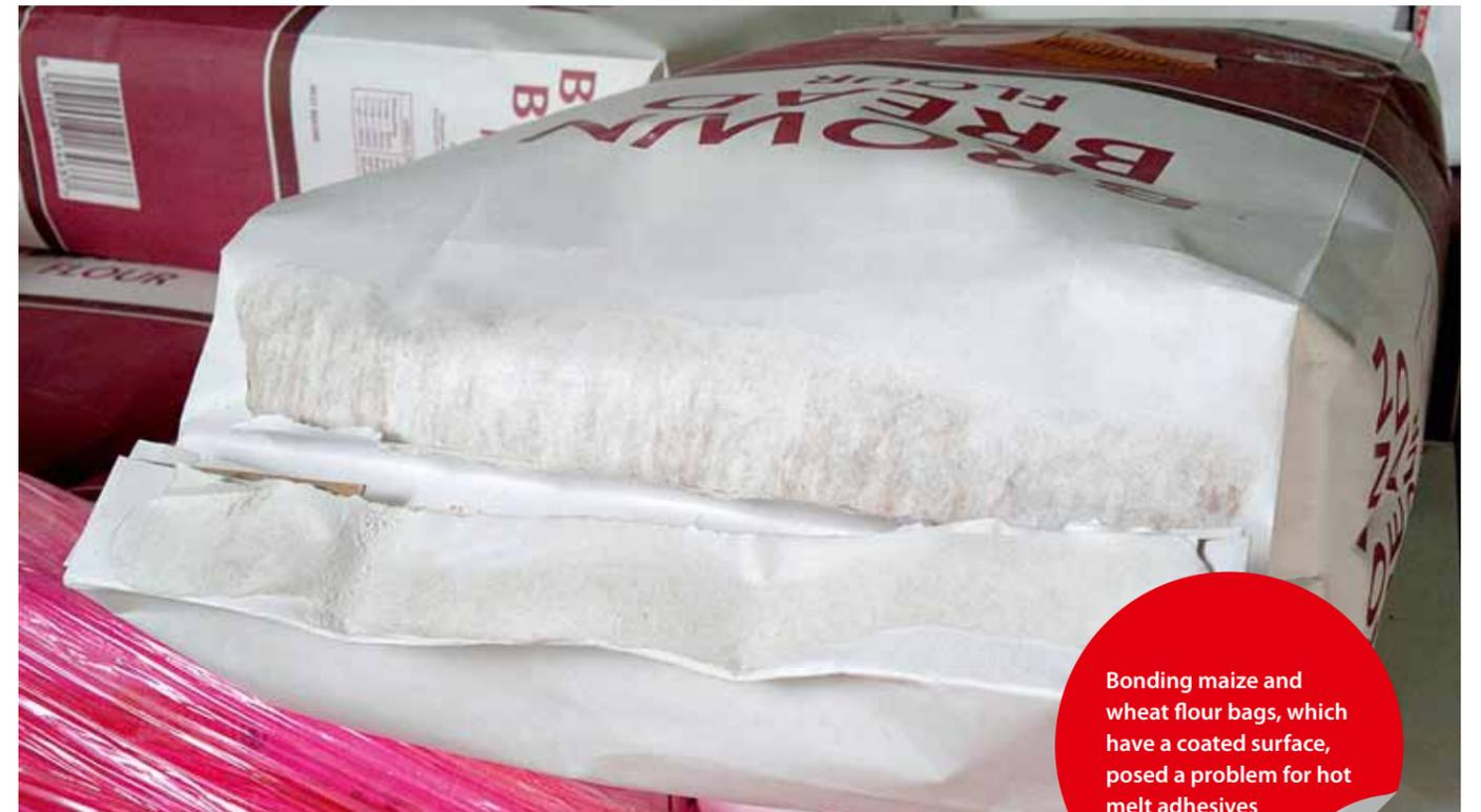
Bonding maize and wheat flour bags, which have a coated surface, posed a problem for hot melt adhesives
