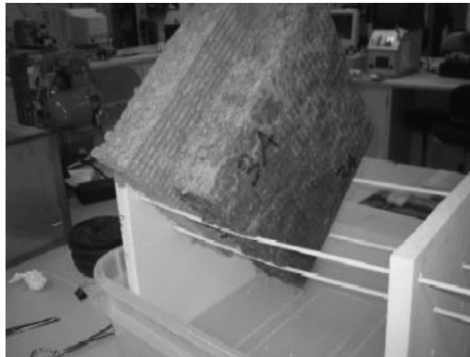
Mineral wool samples drain on edge after 2 hours submerged in water.
