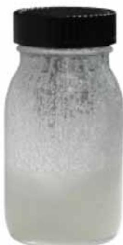
Crystallized liquid epoxy resin
