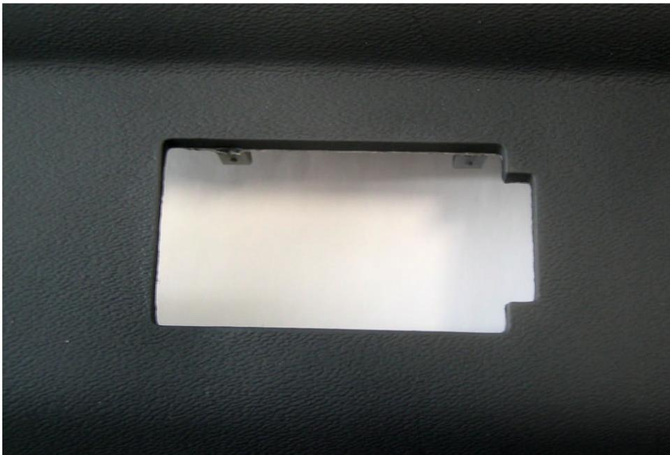
Fig. 5- Same trim part molded with Advanced Reinforced Elastomer (no knit lines).
