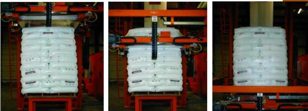
The stretch hood packaging process is fast and efficient, with a throughput of approximately 200 loads per hour (compared to 60-80 loads per hour using stretch wrap).
