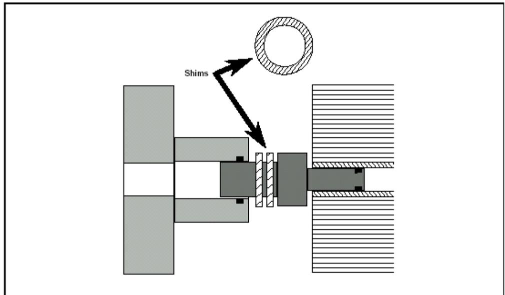
Shims can be purchased from your pressure vessel manufacturer. An alternative is to cut shims from an appropriately sized piece of polyvinylchloride (PVC) pipe. If cut from pipe, the shims must be free of burrs and must be cut parallel and flat to work correctly.
