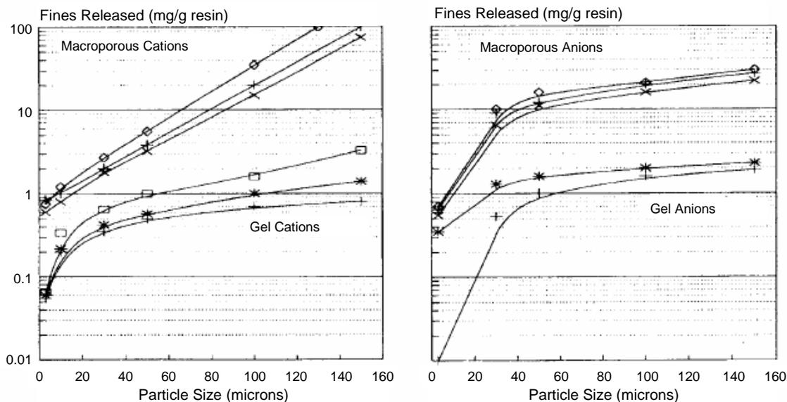
By using gel resins with uniform particle size, the additional advantages of higher operating capacities and better regenerability are combined with optimum separation and minimum cross contamination and osmotic damage.
