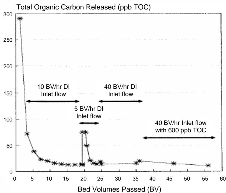
The release of TOC from the resin under these extreme conditions was in the 10 ppb range, indicating excellent resin performance.
