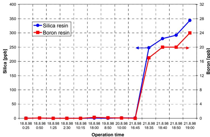
Figure 4. Boron and silica breakthrough at outlet train 2 cation/anion exchanger
