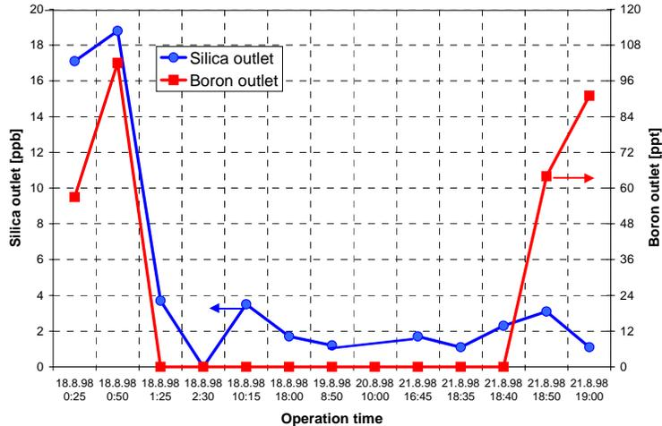
The data collected during start-up in 1998 under normal operating conditions showed that almost no boron (50–100 ppt) was detected in the effluent of the single-bed IX train. Later data showed a stable boron level of <30 ppt in the outlet of the IX train. The first two data sets show the fast rinse phase conditions prior to the train being set into operation.
