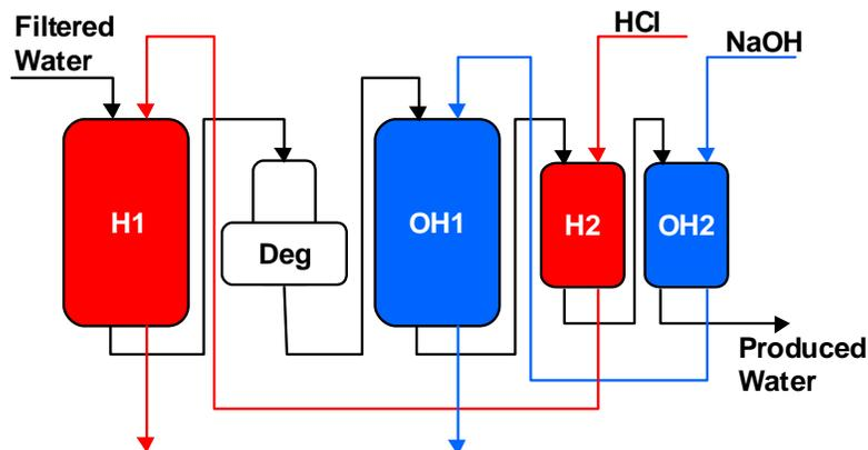
Figure 3. Configuration of the UPCORE™ 4B5T system
