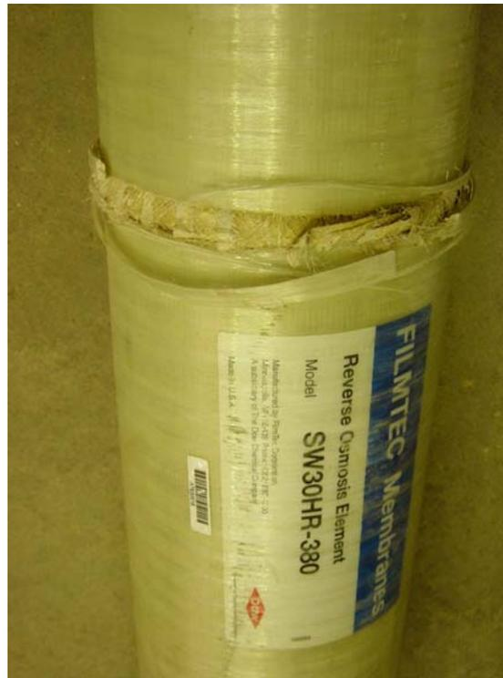
Figure 8.11 High pressure drop due to biofouling has pushed out the feed spacer
