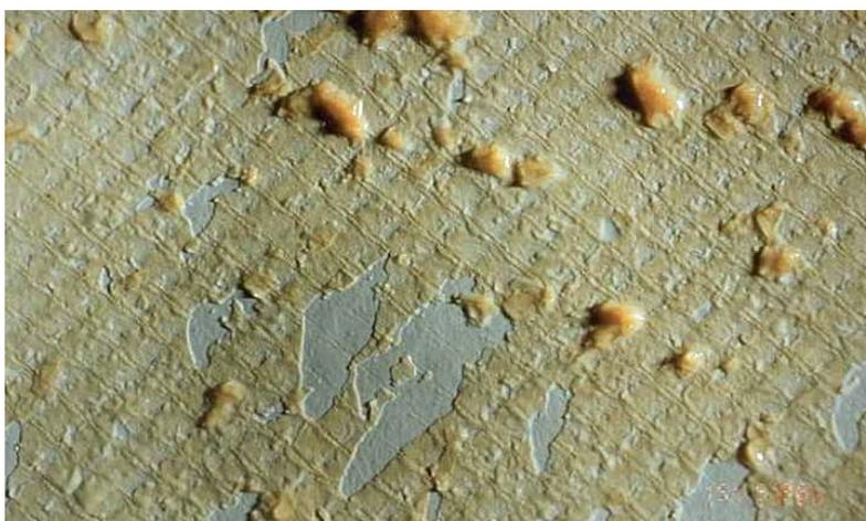
Figure 8.5 Picture of feed spacer with biofilm
