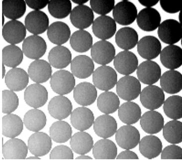
Dow's commercially available Boron Selective Resin, XUS-43594.00 can be applied to remove and reduce boron levels over a wide range of applications, including industrial, agricultural and for high quality drinking water.
