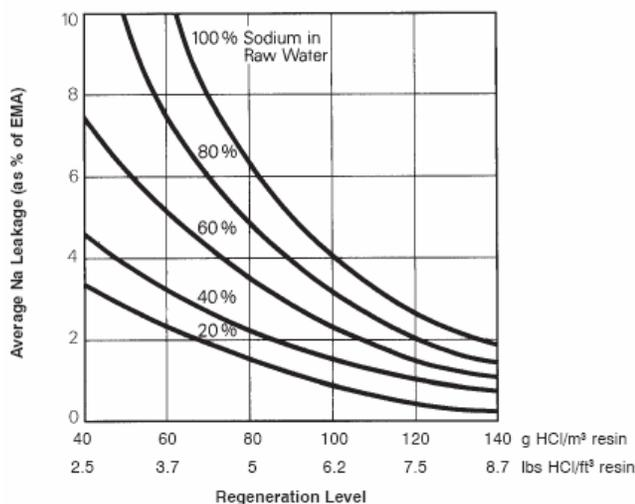
**Figure 7. Average Na leakage from DOWEX HCR-W2 and DOWEX HGR-W2 resins in co-current operation with H<sub>2</sub>SO<sub>4</sub> as regenerant**
