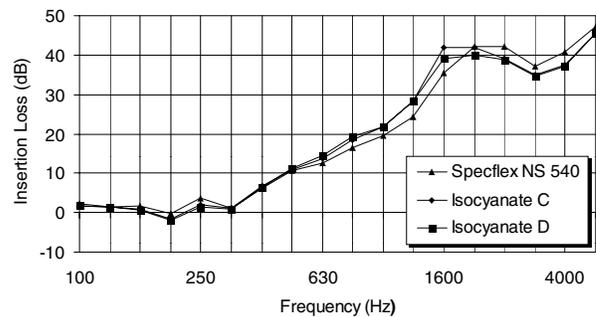
Figure 10: Petite Cabine IL of foams based on Polyol D
