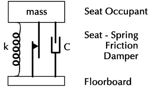
Figure 1: Damped harmonic oscillator model for seat performance
