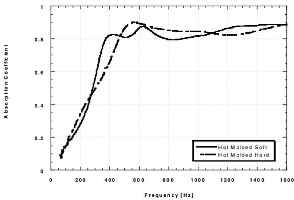
Figure 6: Effect of Hardness on Sound Absorption
