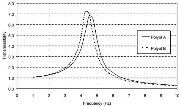
Figure 3: Vibration Curves (MTS test) for TDI/MDI (TM20) HR Foams (Polyols A & B)
