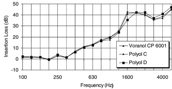
Figure 9: Petite Cabine IL of foams based on SPECIFLEX NS 540
