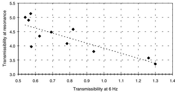
Figure 2: Effect of the Transmissibility at resonance ( $a_r$ ) on the Transmissibility at 6 Hz (TDI/MDI based foams, density:  $50 \text{ kg/m}^3$ , hardness:  $20\text{-}22 \text{ kgf/314 cm}^2$  at 25% indentation) in the JASO test.
