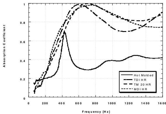
Figure 7: Sound Absorption for 60mm thick samples with skin
