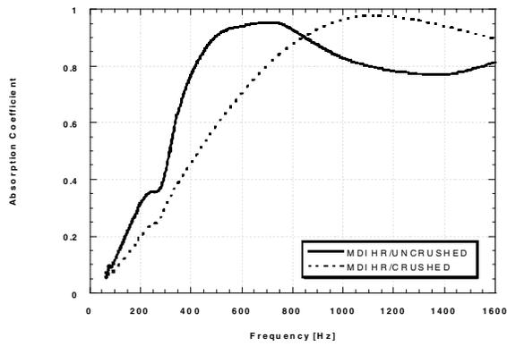
Figure 5: Effect of Crushing on Sound Absorption
