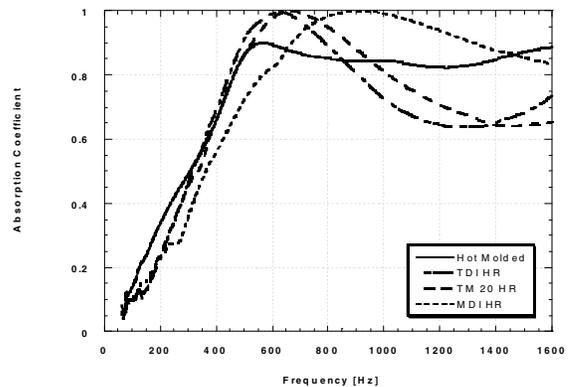
Figure 4: Sound Absorption for 60mm thick core samples
