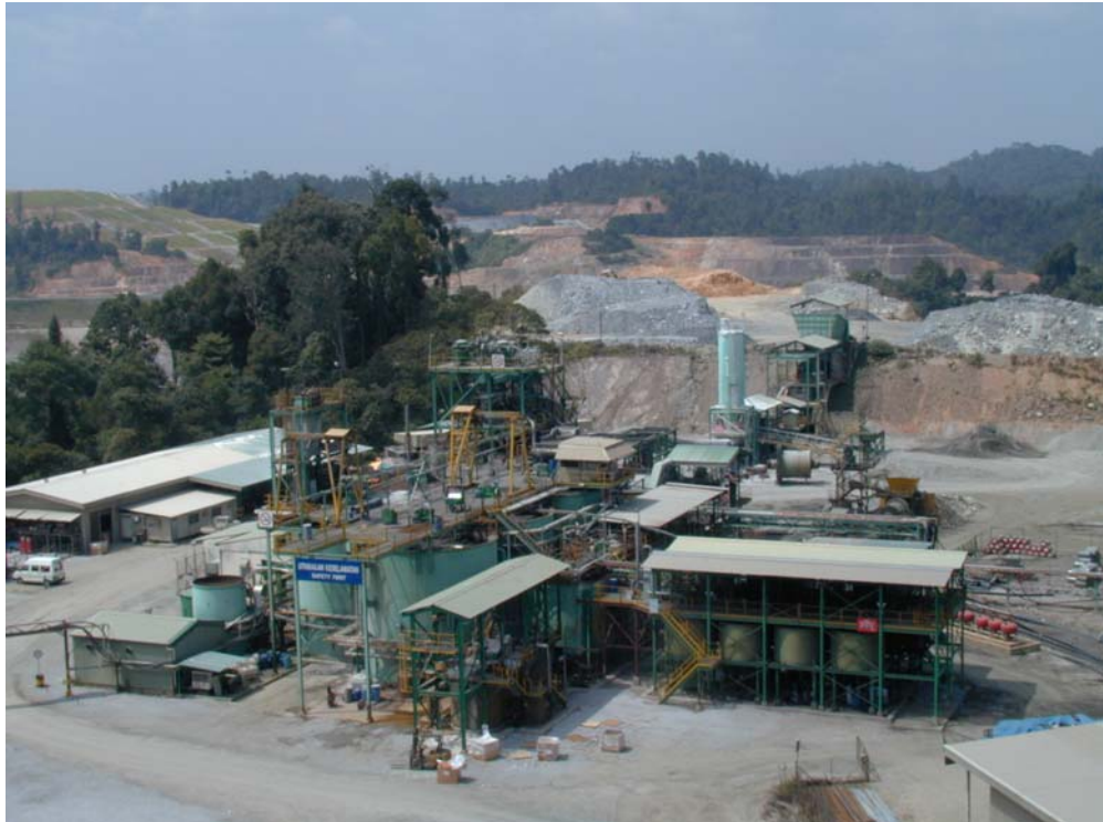
Avocet Mining's Penjom gold mine uses a Dow developmental gold-selective resin to boost gold recovery from carbonaceous ore. (Photo courtesy of Avocet Mining)
