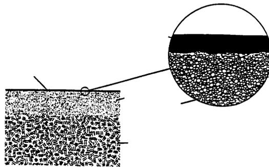
Polyamide, Microporous Polysulfone, Polyester Support Web, Ultrathin Barrier Layer
