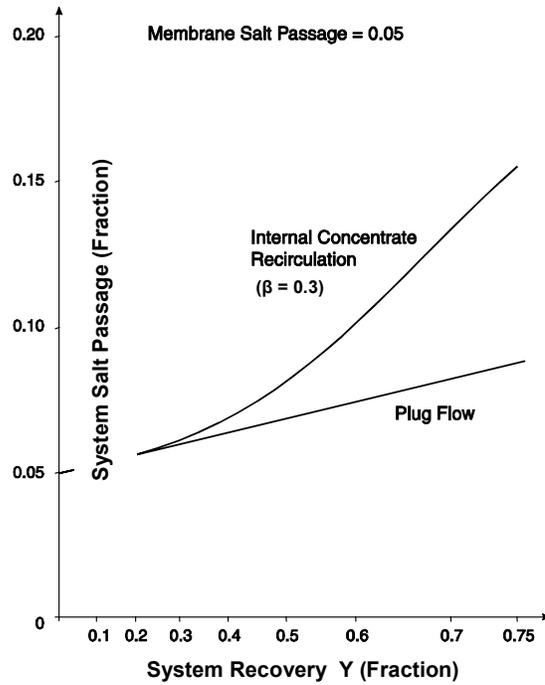
When the recirculated concentrate stream approaches zero, the  $\beta$  number approaches  $1/[(1/Y) - 1]$ , and the recirculation system becomes a plug flow system. A compromise between plug flow and recirculation systems is the tapered recirculation system with a declining number of parallel modules per stage when viewed in feed flow direction (see Figure 3.8).
