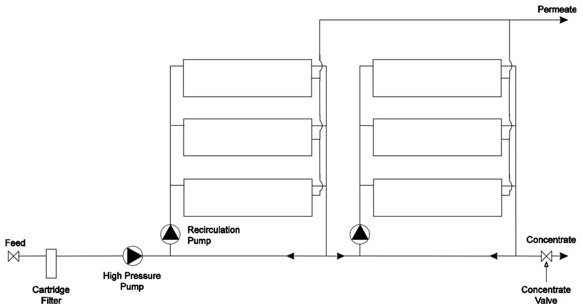
The main advantage of the recirculation concept is the defined feed flow rate to the modules regardless of the degree of fouling of preceding modules and the changes in feed water composition. Further aspects of the recirculation concept are mentioned in [Batch vs. Continuous Process \(Section 3.2\)](#), and [Single-Module System \(Section 3.3\)](#). A comparative summary is given in Table 3.3.
