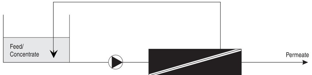
The semi-batch mode is a modification of the batch mode. In semi-batch mode of operation the feed tank is refilled with feed water already during operation. The batch is terminated with the feed tank full of concentrate. This allows a smaller tank to be used.
