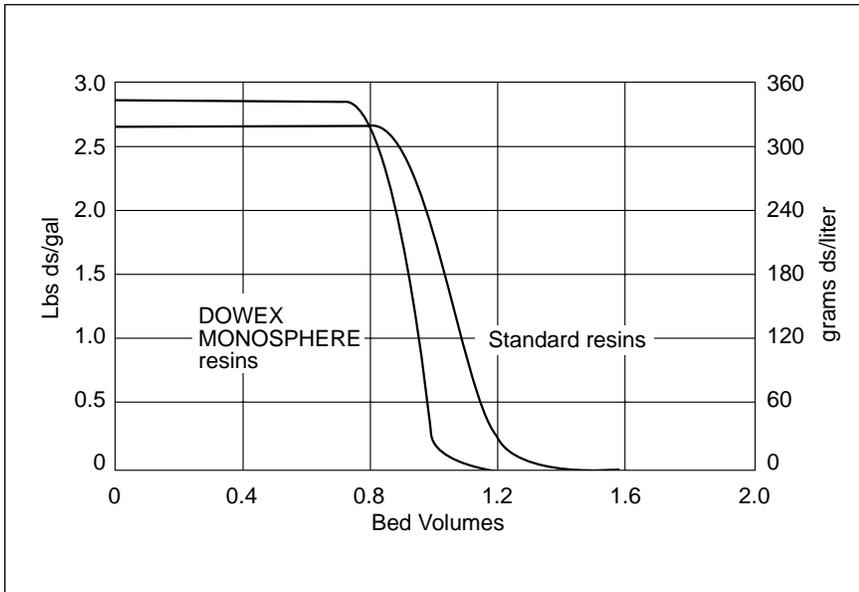
This graph tracks the dextrose side cation-anion effluent during sweetening-off. Notice the shorter, steeper profile of DOWEX MONOSPHERE resins. More efficient rinsing and longer service cycles each lead to significant reductions in sweetwater and wastewater.
