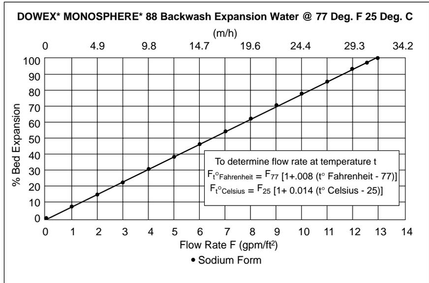
**Figure 23 – Backwash expansion of DOWEX 88 resin**
