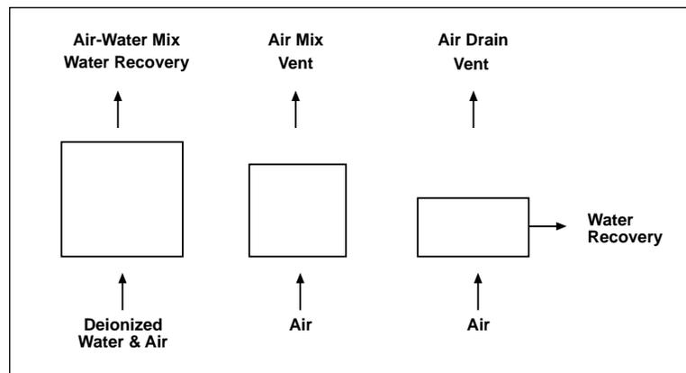
**Figure 11– Recycle rinsing of mixed beds**
