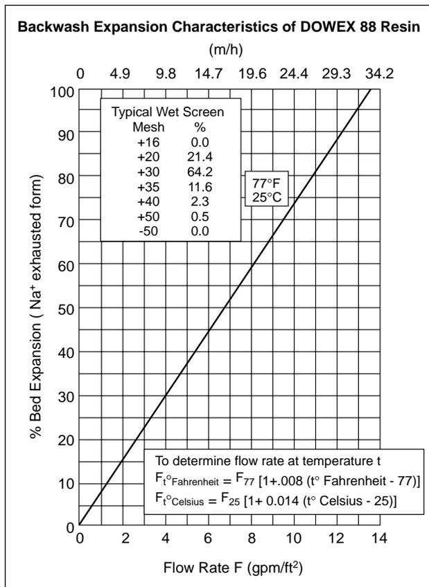
**Figure 25 – Backwash expansion of DOWEX 66 resin**
