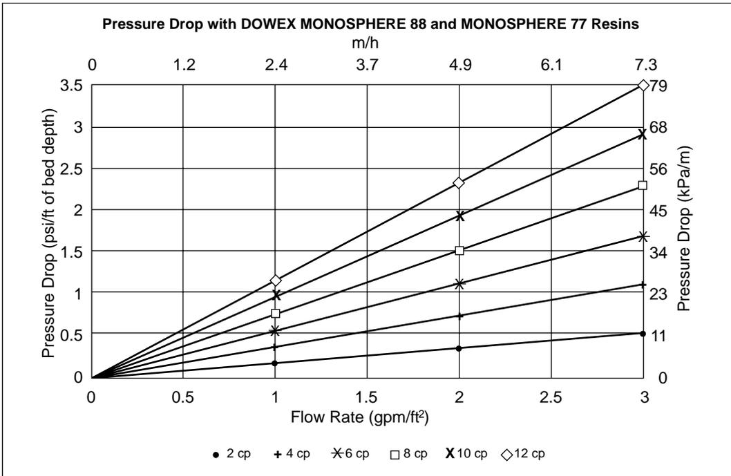
Figure 21 – Pressure drop with DOWEX 88 MB resin
