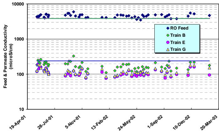
Figure 4. Averaged rejection data for three trains with new elements.
