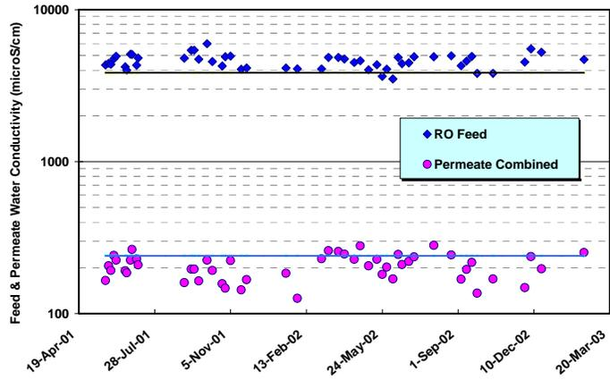
Figure 3. Conductivity of RO feed and permeate from three trains with new elements from April 2001 to March 2003.
