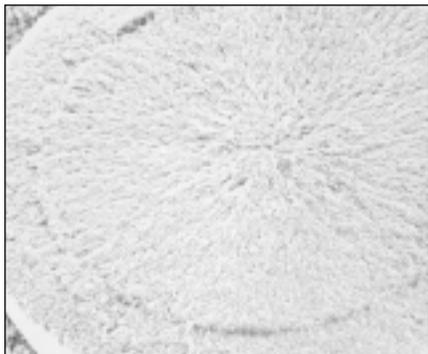
This cross section of a DOWEX macroporous ion exchange bead shows the countless tiny pores through which syrup components diffuse. This structure permits maximum syrup contact with the polymer's functional sites while providing the physical strength required for long life.
