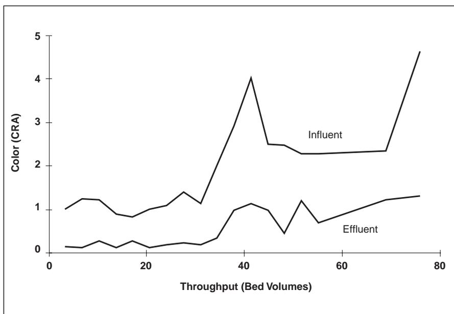
**Figure 5. Removal of After-Heat Color from Corn Syrup Single-Pass**
