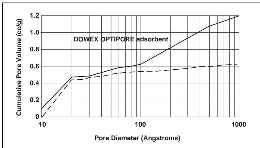
ion exchange resins, the adsorbent has a minimal amount of ion exchange capacity and instead depends upon adsorption for the removal of color bodies. DOWEX OPTIPORE SD-2 adsorbent was specially designed to mimic the porosity found in activated carbon in the range of pore sizes critical for color component adsorption (Figure 1). The large amount of porosity greater than 100 Å allows for fast kinetics.
