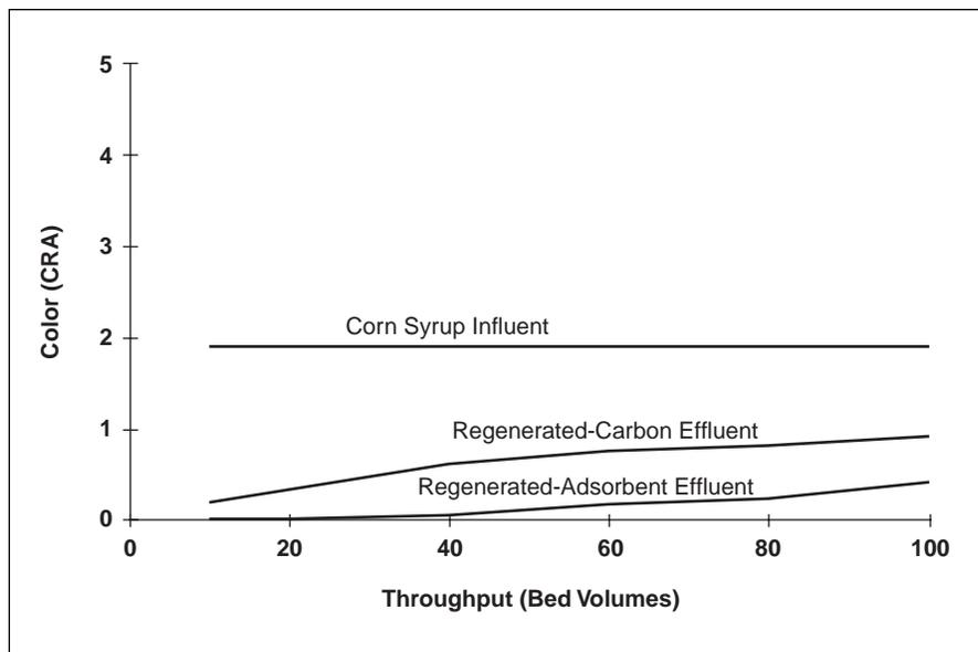
**Figure 3. Comparison of DOWEX OPTIPORE Adsorbent and Activated Carbon - After-Heat Color**
