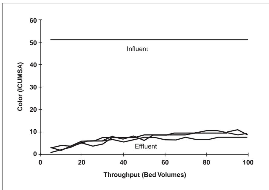
Color and heat-color removal capabilities are again comparable to those obtained with activated carbon, when the resin is used on the fructose side of the HFCS process. An approximately 70-75% reduction in color is obtained as well as a 50% reduction in after-heat color (Figures 8 and 9). The synergistic effect of DOWEX OPTIPORE SD-2 adsorbent with ion exchange resin on the reduction of after-heat color has also been demonstrated.
