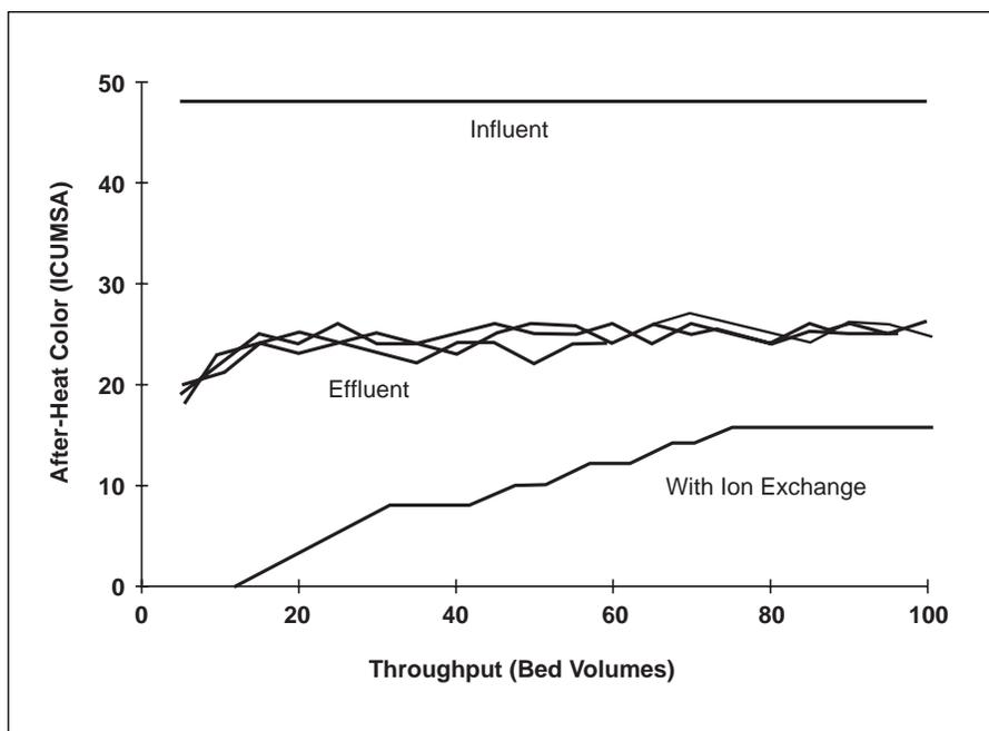
An added benefit of using DOWEX OPTIPORE SD-2 adsorbent in fructose service is the removal of HMF. DOWEX OPTIPORE SD-2 is very effective at removing HMF from HFCS during the early portion of its cycles. At 65 bed volumes of throughput, or approximately 22 hours of cycle time, the adsorbent has removed at least 50% of the HMF in the syrup stream (Figure 10).
